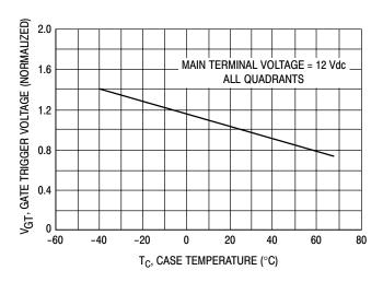
Figure 5. Typical Gate Trigger Voltage
