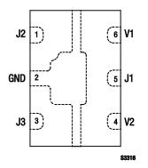
Figure 2. SKY13290-313LF Pinout –6-Pin QFN (Top View)
