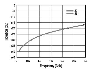
**Figure 4. Isolation vs Frequency**
