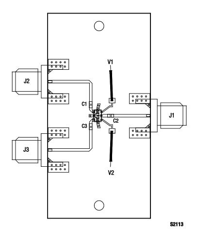
Figure 8. SKY13290-313LF Evaluation Board Assembly Diagram
