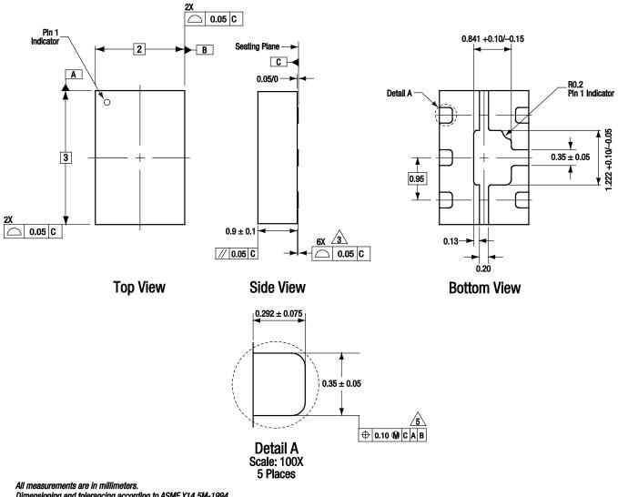
Dimensioning and tolerancing according to ASME Y14.5M-1994. Coplararity applies to the terminals and all other bottom surface metalization. Dimension applies to metalized terminal. If the terminal has a radius on its
