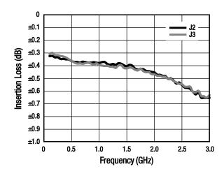
**Figure 3. Insertion Loss vs Frequency**
