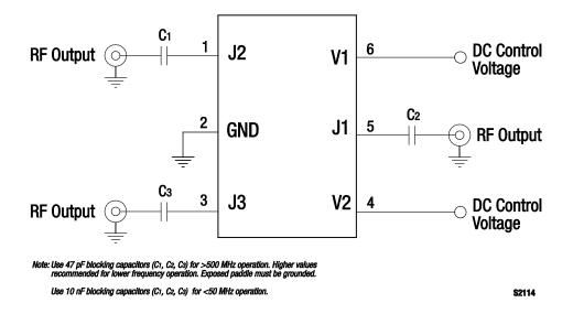
Figure 7. SKY13290-313LF Evaluation Board Schematic
