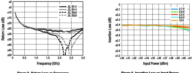
Figure 5. Return Loss vs Frequency (Insertion Loss State)
