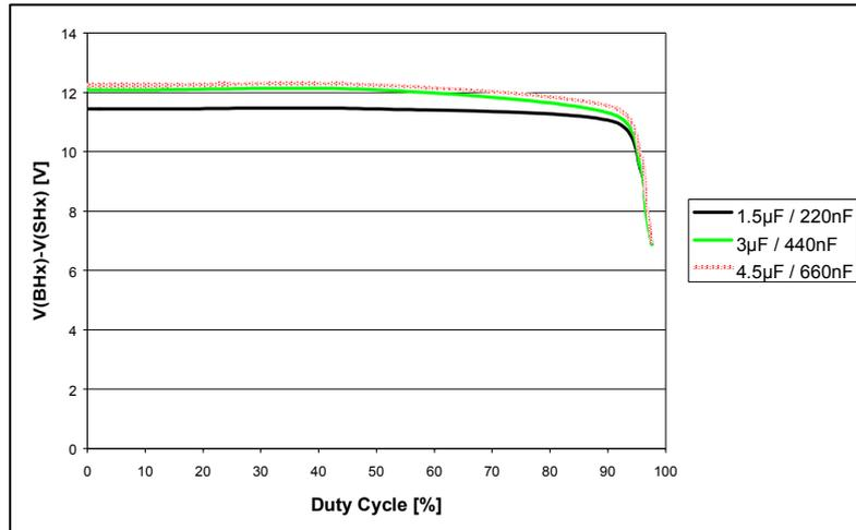
**Fig. 13: Typ. bootstrap voltage  $V(BHx)-V(SHx)$ ; duty cycle of 1 half-bridge = 50%; duty cycle of the other 2 halfbridges variable**
