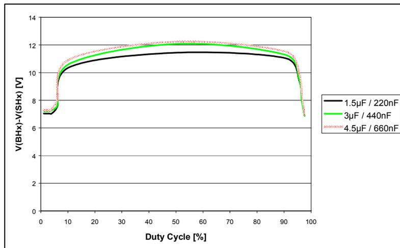
**Fig. 14: Typ. bootstrap voltage  $V(BHx)-V(SHx)$ ; duty cycle of 1 half-bridge = 0%; duty cycle of the other 2 halfbridges variable**
