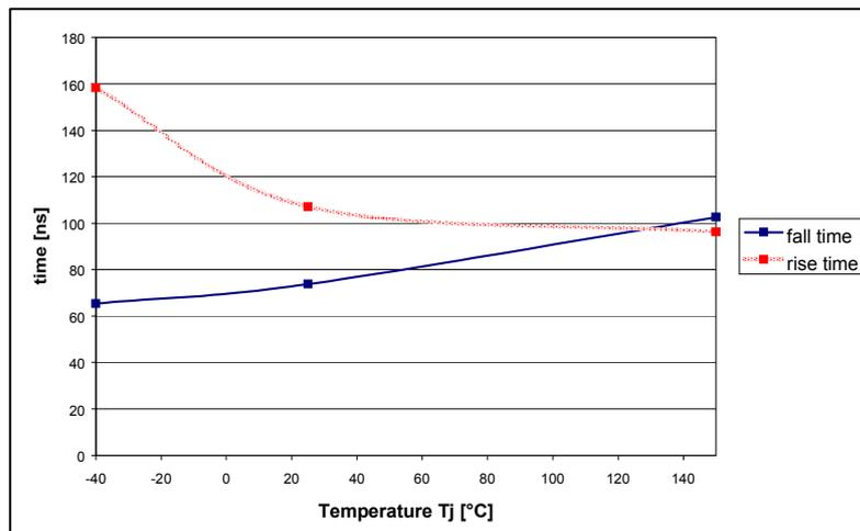
**Fig. 19: Rise- and fall-times vs. temperature T<sub>J</sub>**
