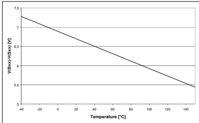
**Fig. 11: Typ. undervoltage shut down (Voltage of bootstrap capacitors)**
