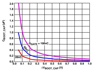
FIGURE 4. BOOTSTRAP CAPACITANCE vs BOOT RIPPLE VOLTAGE
