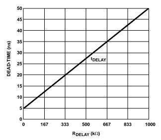
FIGURE 3. ISL6210 PROGRAMMABLE DEAD-TIME vs DELAY RESISTOR
