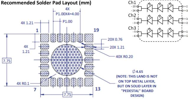
Figure 2a: Recommended solder pad layout for anode, cathode, and thermal pad.
