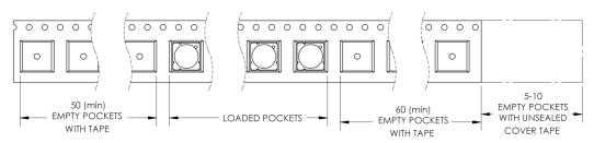
Figure 11: Emitter carrier tape specifications (mm).
