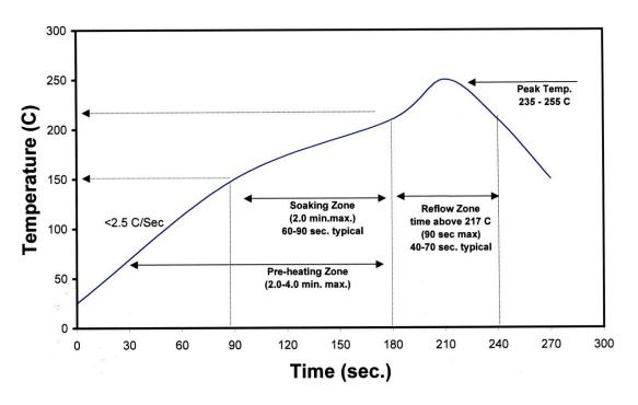
Figure 3: Reflow soldering profile for lead free soldering.
