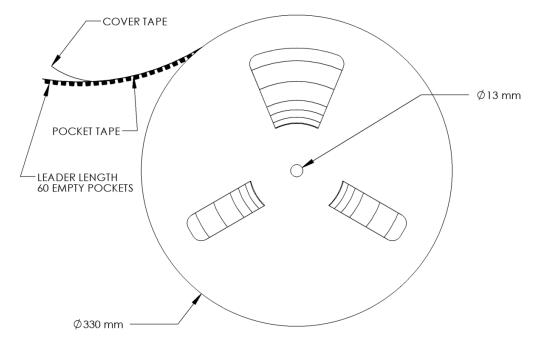
Figure 12: Emitter Reel specifications (mm).
