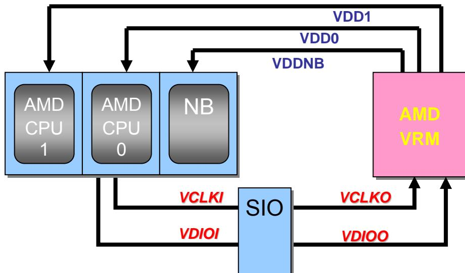
AMD SVID use *smbus* to transmit serial data VCLK and VDIO, thus its max speed can up to 400KHz. We support 4 mode (Bypass; offset; manual; compare) liked as PVID, and we can control output frequency according *Factor\_L* and *Factor\_M* register.
