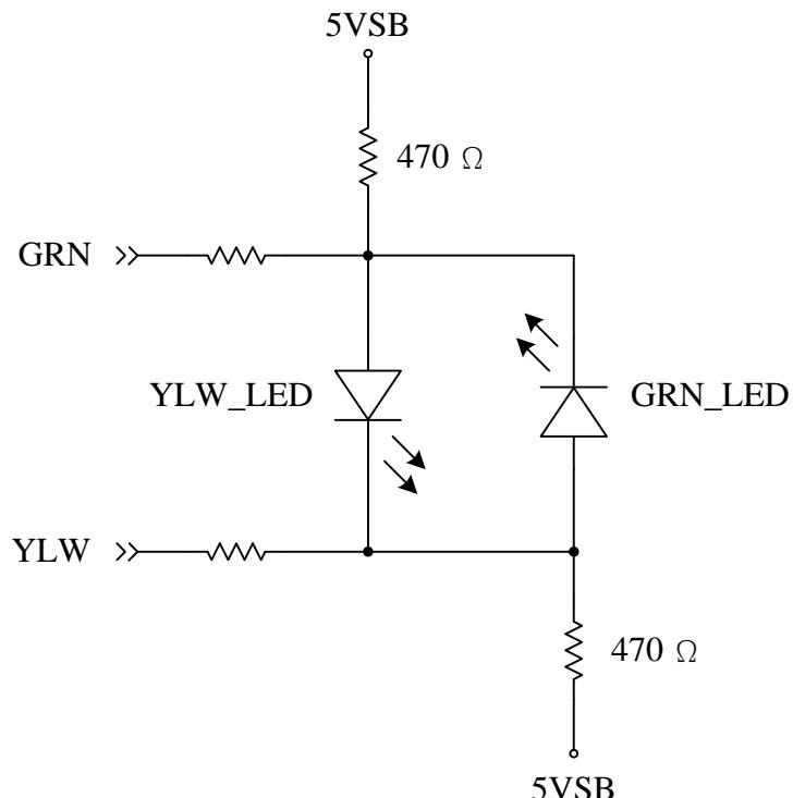
Figure 6-9 Illustration of Dual Color LED application
