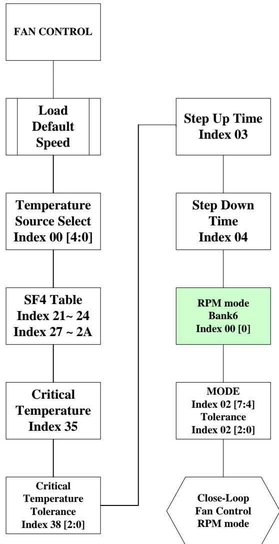
Figure 8-15 Close-Loop Fan Control RPM mode Programming Flow
