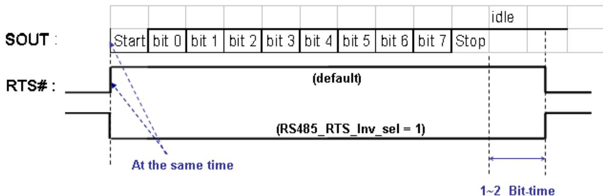
The default behavior of RTS# pin will drive logic high the time edge between **Start bit** and **bit0** when the UART TX Block start to transmits the data on SOUT pin. Then the RTS# pin will drive logic low later than **Stop bit** about 1~2 x Bit-time when UART TX Block completes the data transmission. The driving behavior of RTS# will be inverted when we set RS485\_RTS\_inv\_sel bit = 1'b1. (Bit-time: Depends on the baud rate of transmission)
