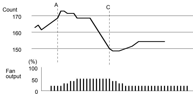
Figure 8-12 Mechanism of Fan Speed Cruise™ Mode
