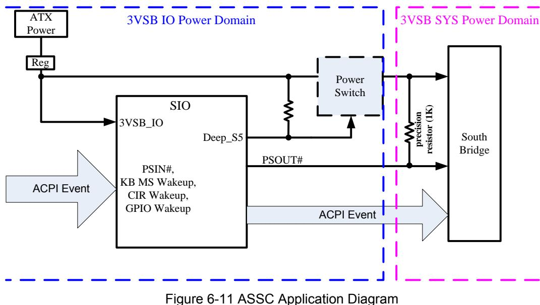
Figure 6-11 ASSC Application Diagram
