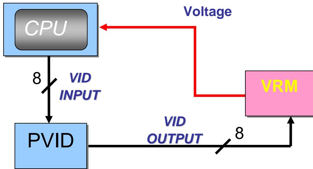
VID input is decoded by SIO according VID table to VID output , and fed to VRM .
