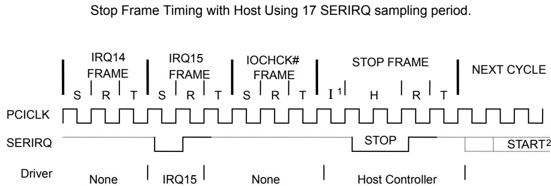
Figure 17-2 Stop Frame Timing with Host Using 17 SERIRQ Sampling Period
