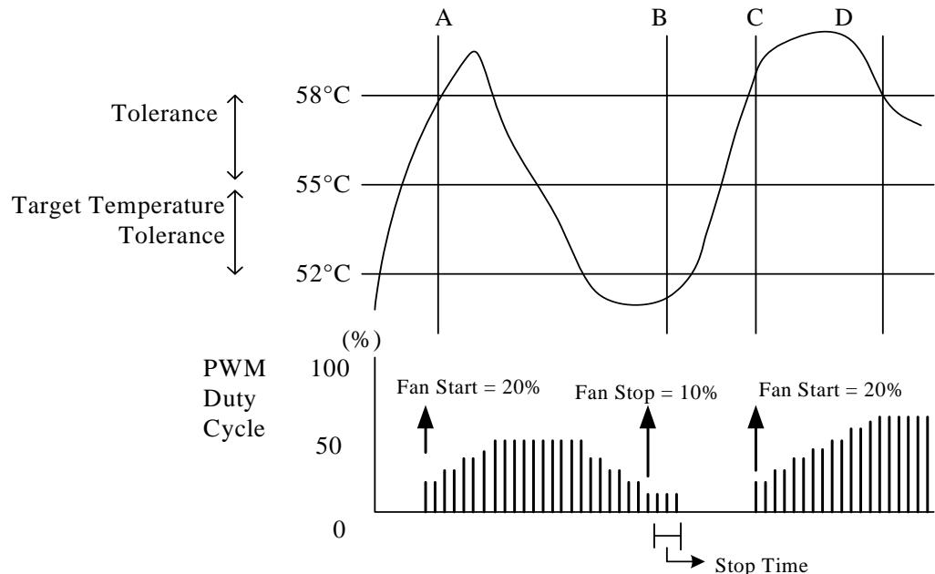
Figure 8-10 Mechanism of Thermal Cruise™ Mode (PWN Duty Cycle)
