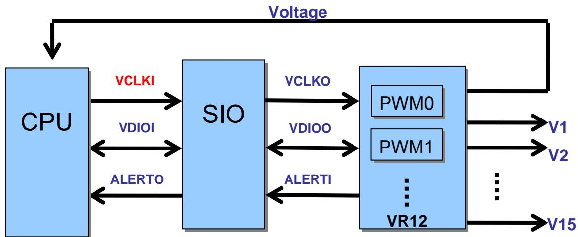
Intel Serial VID use *pmbus* to transmit serial data SVC and SVD, thus its max speed can up to 33MHz. We support 4 mode (Bypass; offset; manual; compare) liked as Parallel VID.
