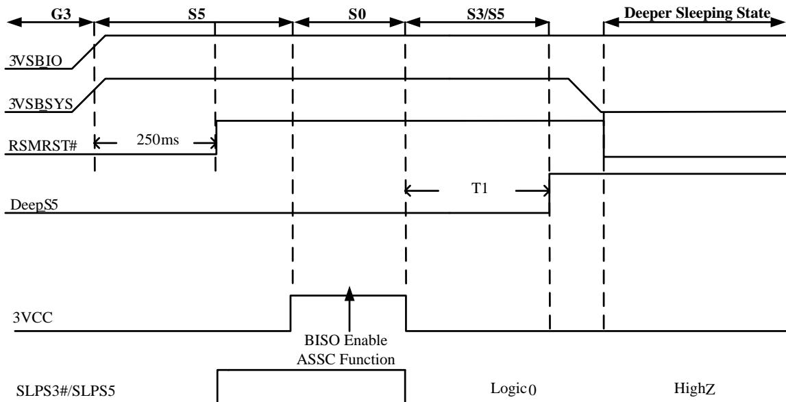
When the first time AC plug in and enter into S0 State, BIOS can enable ASSC Function (DeepS3 or DeepS5), when the system enters S3/S5 state, the pin DEEP\_S5 will be asserted after pre configuration delay time (power\_off\_dly\_time, LD16 CRE2) to make the system entering the “Deeper Sleeping State (DSS)” where system’s VSB power is cut off. When pin DEEP\_S5 asserts, the pin RSMRST# will de-assert by detecting PSOUT# signal (monitor 3VSB SYS Power).
