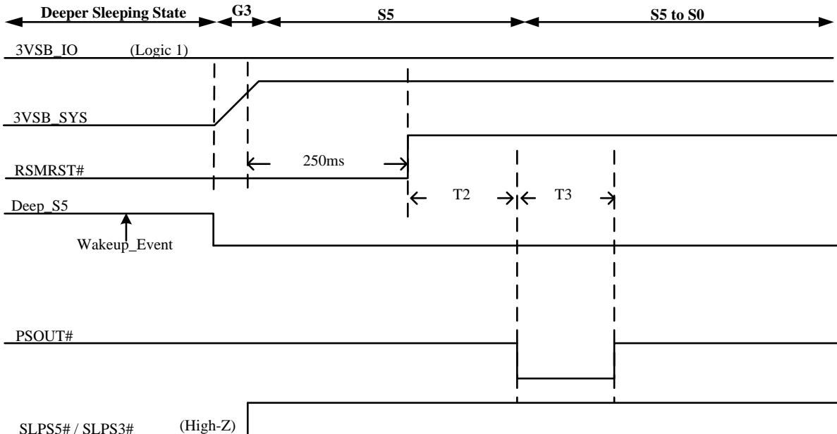
When any Wakeup Event (PSIN#, KB MS Wakeup, CIR wakeup, GPIO Wakeup) happened, pin DEEP\_S5 will be de-asserted to turn on the VSB power to the system. The pin RSMRST# will de-assert when 3VSB\_SYS power reach valid voltage. And then the pin PSOUT# will issue a low pulse (T3) turn on the system after T2 time (wakeup delay time, LD16 CRE0). The PSOUT# low pulse is also programmable (LD16 CRE1). The T4 time is the delay from Deep\_S5 ds-assert to Deep\_S5#\_DELAY de-assert.
