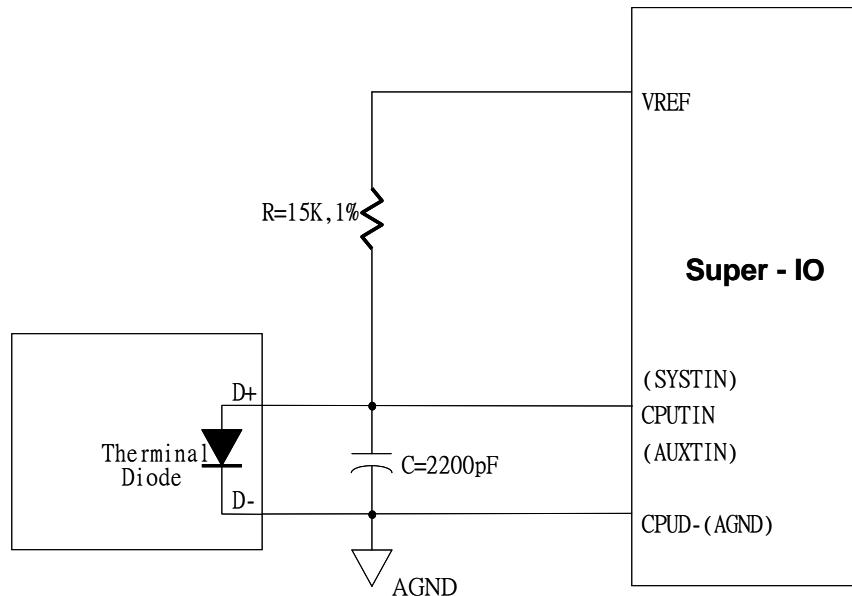
Figure 8-6 Monitoring Temperature from Thermal Diode (Voltage Mode)
