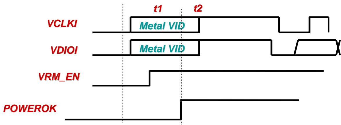
AMD SVID has two table, one is metal VID table and another is Serial table. When VRM\_EN = 1 (**t1**), VRM should look up metal VID table to decode. After a while (**t2**), as CPU send Serial Code, VRM should look up serial table.
