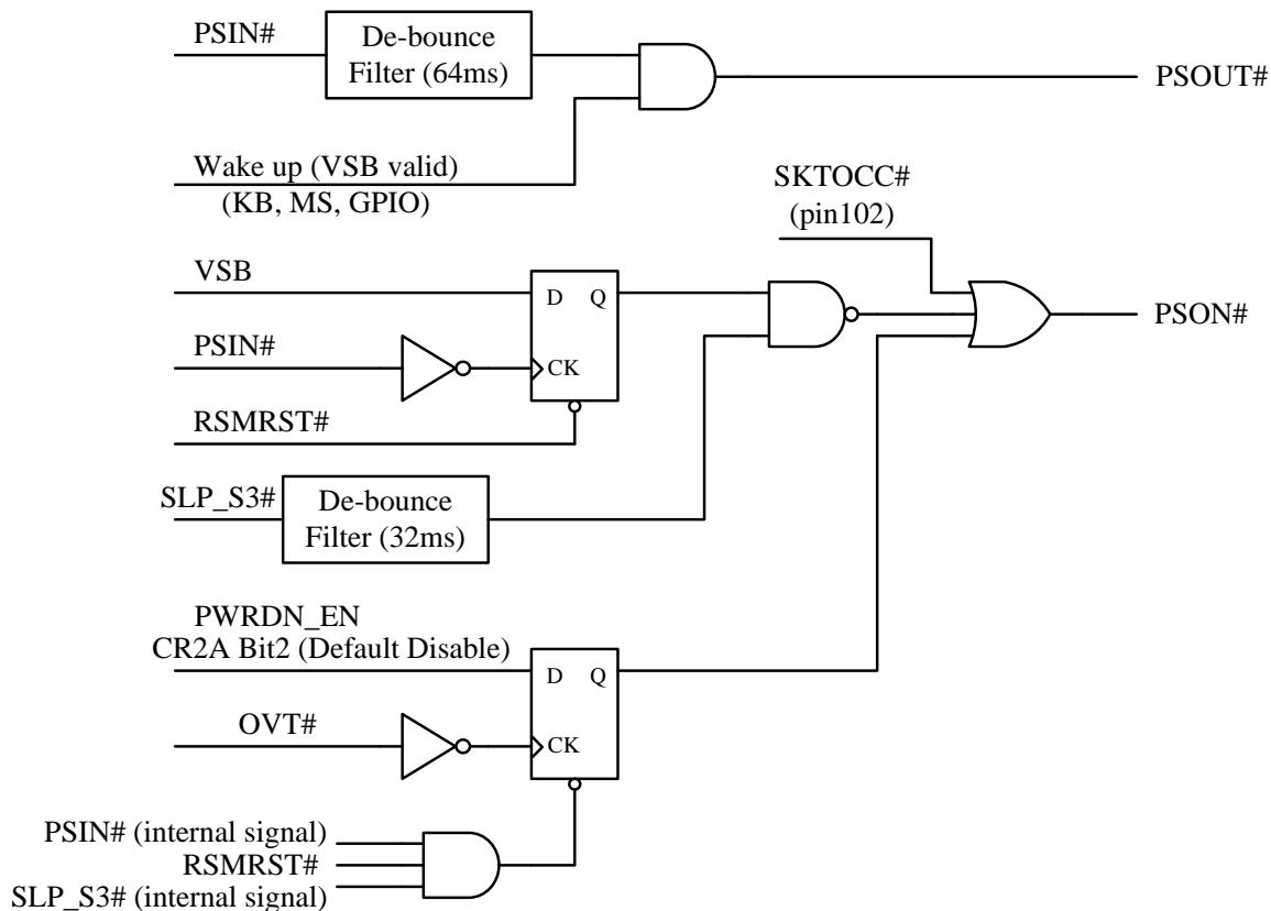
Figure 6-7 PSON# Block Diagram
