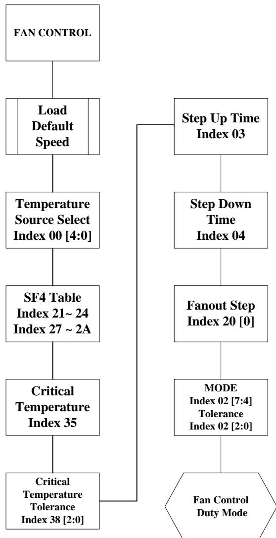
Figure 8-14 Fan Control Duty Mode Programming Flow
