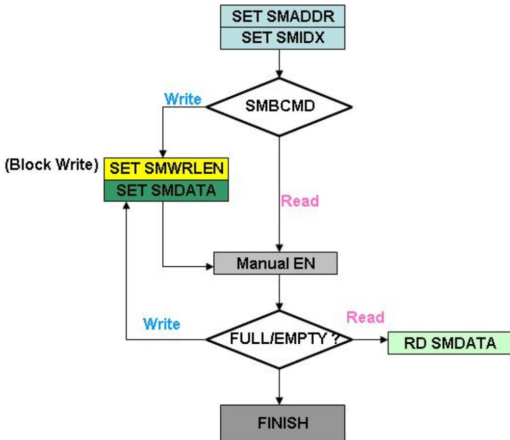
Figure 23-9 Manual Mode Programming Flow
