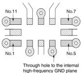
• Connect each high-frequency GND pad to the internal high-frequency GND plane through the through holes.
