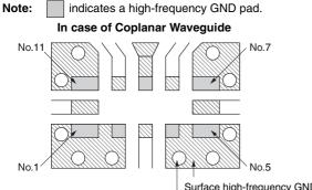
Surface high-frequency GND plane Through hole to the internal high-frequency GND plane
