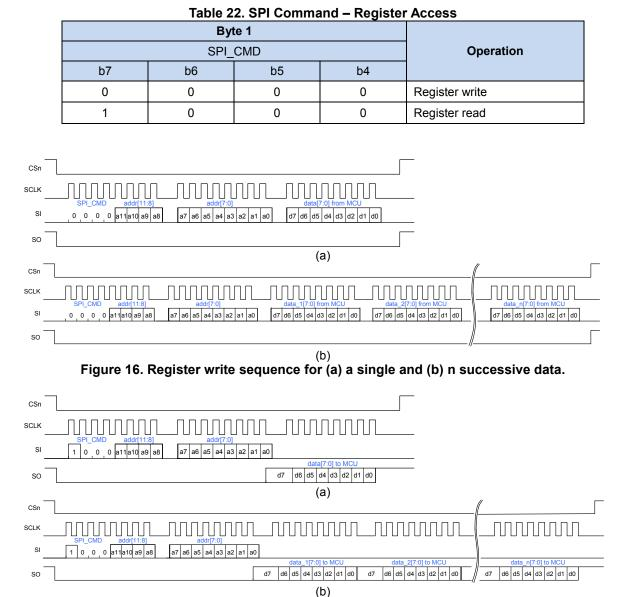
Figure 17. Register read sequence for (a) a single and (b) *n* successive data.
