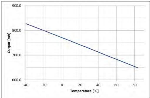
Figure 13. Temperature sensor output voltage.
