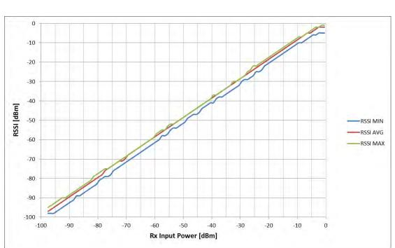
Figure 10. Typical RSSI value vs. RX input power for 250kbps.
