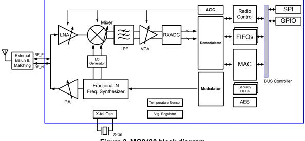
Figure 3. MG2420 block diagram.
