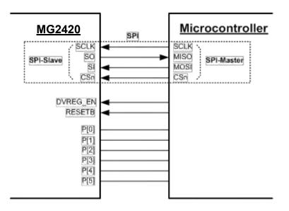
Figure 14. Microcontroller to MG2420 interfaces.
