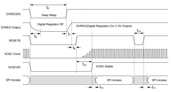
Figure 20. RESETB and DVREGEN signal diagram
