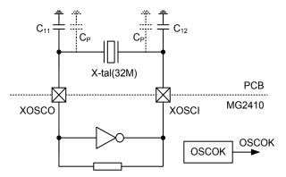
Figure 12. Simplified Crystal Oscillator schematic.
