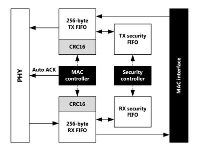
Figure 11. Integrated MAC structure
