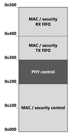
Figure 23. Overall register address space
