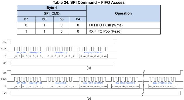
Figure 18. TX FIFO write sequence. (a) Single and (b) Multiple data access.
