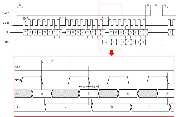
Figure 15. SPI timing diagram.
