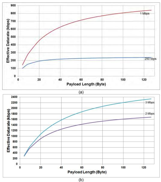
Figure 9. Effective payload data rate. (a) 2Mcps mode. (b) 4Mcps mode.
