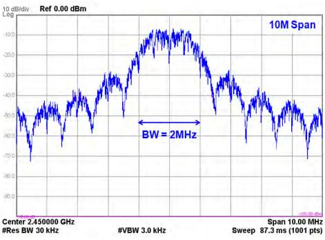
Figure 5. Modulated signal spectrum for 2Mcps mode.
