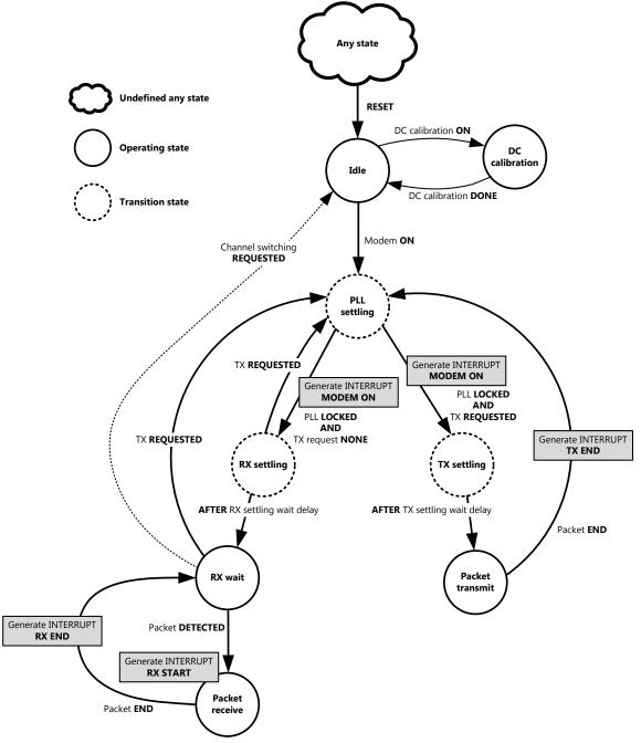
Figure 22. Basic MG2420 State Transition Diagram
