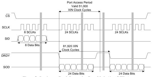
Figure 5. Continuous Read Conversion Data Mode (4 or 5 Wire)
