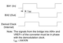
Figure 8. External Excitation Clock Phasing
