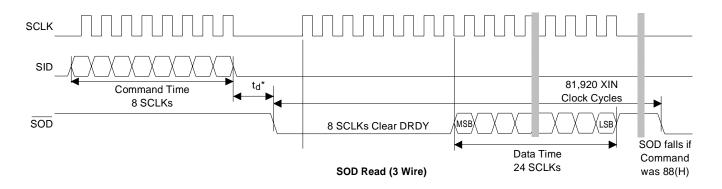
Figure 4. Command and Data Word Timing
