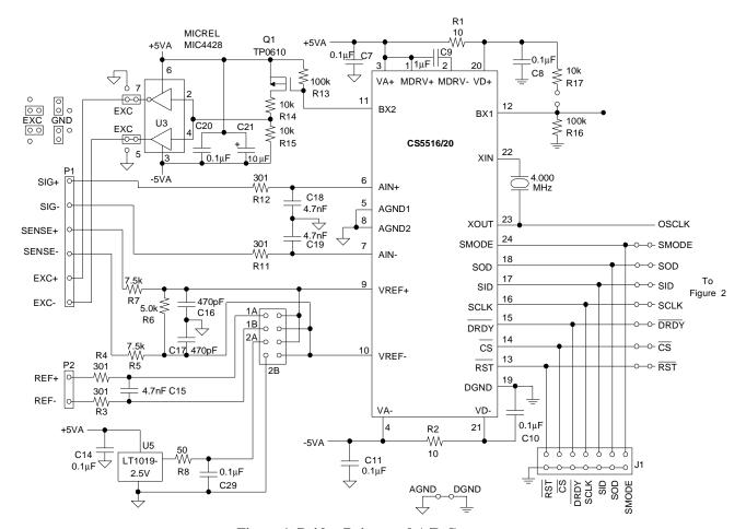
Figure 1. Bridge Driver and A/D Converter
