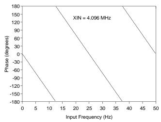
Figure 12. Filter Phase Response.
