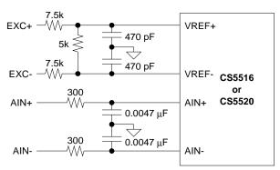
Figure 9. AIN and VREF Input Filter Components
