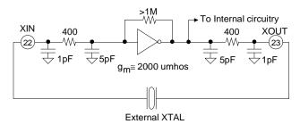
Figure 10. On-Chip Gate Oscillator Model
