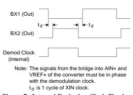
Figure 7. Internal Excitation Clock Phasing
