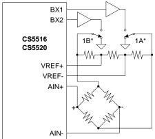
\*Note: The bridge can be grounded with a relay or with jumpers to perform non-ratiometric calibration.
