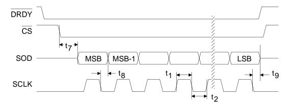
**SOD Read Timing (Not to Scale)**
