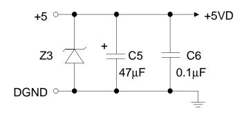
Figure 6. Using Off-board Voltage Reference
