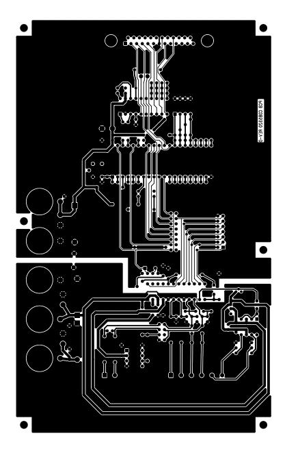
Figure 10. CDB5520 Solder Side Trace Layer
