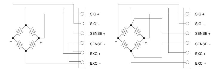
Figure 4. 4-Wire Bridge Connections
