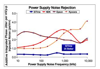
Figure 4. Power Supply Noise Rejection<sup>[4]</sup>
