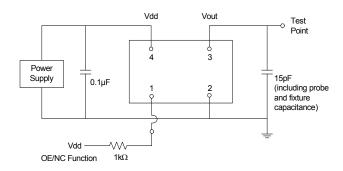
Figure 2. Test Circuit
