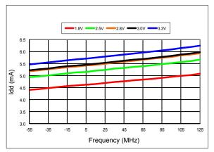
Figure 7. Idd vs Frequency
