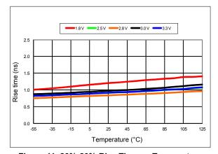
Figure 11. 20%-80% Rise Time vs Temperature
