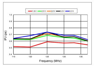
Figure 14. RMS Integrated Phase Jitter Random (900 kHz to 7.5 MHz) vs Frequency<sup>[11]</sup>
