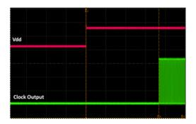
Figure 16. Startup Waveform vs. Vdd
