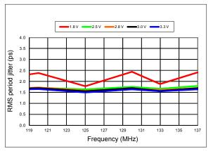
Figure 9. RMS Period Jitter vs Frequency
