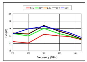
Figure 13. RMS Integrated Phase Jitter Random (12k to 20 MHz) vs Frequency<sup>[11]</sup>
