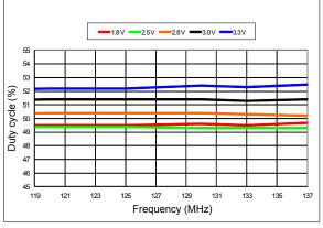
Figure 10. Duty Cycle vs Frequency
