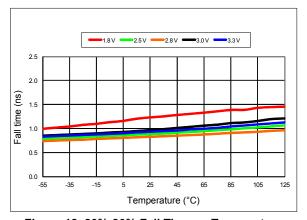
Figure 12. 20%-80% Fall Time vs Temperature
