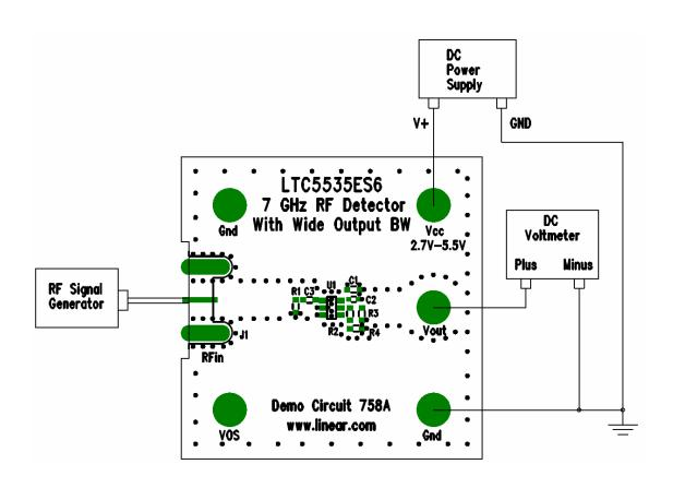
Figure 1. Proper Measurement Equipment Setup
