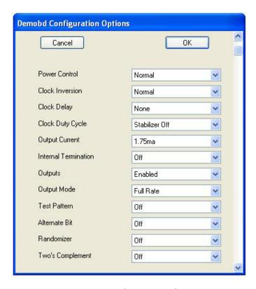
Figure 4. Demobd Configuration Options
