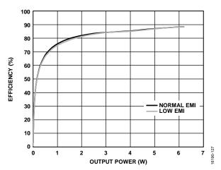
Figure 33. Efficiency vs. Output Power ( $P_{OUT}$ ),  $R_L = 4 \Omega$ , No Ferrite Bead (FB) and 220pF Capacitor,  $PV_{DD} = 7 V$ , Analog Gain = 8.9
