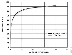
Figure 53. Efficiency vs. Output Power ( $P_{OUT}$ ),  $R_L = 8 \Omega$ , FB and 220 pF Capacitor,  $PV_{DD} = 17 V$ , Analog Gain = 16
