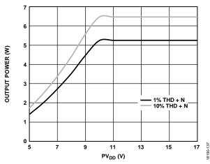
Figure 43. Output Power vs.  $PV_{DD}$  Supply Voltage ( $PV_{DD}$ ),  $R_L = 8 \Omega$ , Analog Gain = 8.9
