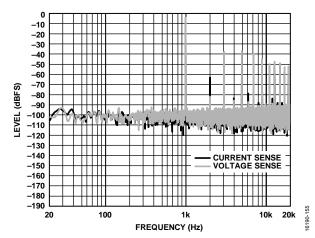
Figure 60. I/V Sense Output FFT, -1 dBFS Input,  $PV_{DD} = 12 V$ , Analog Gain = 12.6
