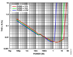
Figure 23. THD + N vs. Output Power,  $R_L = 4 \Omega$ , Analog Gain = 16
