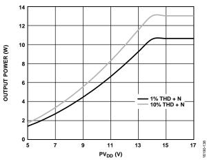
Figure 44. Output Power vs.  $PV_{DD}$  Supply Voltage ( $PV_{DD}$ ),  $R_L = 8 \Omega$ , Analog Gain = 12.6
