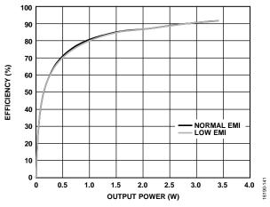
Figure 47. Efficiency vs. Output Power ( $P_{OUT}$ ),  $R_L = 8 \Omega$ , No FB and 220 pF Capacitor, PV<sub>DD</sub> = 7 V, Analog Gain = 8.9
