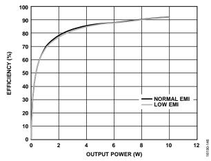
Figure 52. Efficiency vs. Output Power ( $P_{OUT}$ ),  $R_L = 8 \Omega$ , FB and 220 pF Capacitor,  $PV_{DD} = 12 V$ , Analog Gain = 12.6
