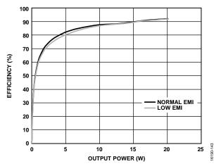
Figure 49. Efficiency vs. Output Power ( $P_{OUT}$ ),  $R_L = 8 \Omega$ , No FB and 220 pF Capacitor,  $PV_{DD} = 17 V$ , Analog Gain = 16
