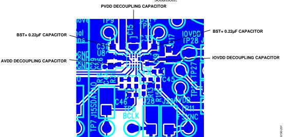
Figure 79. Recommended Component Placement {should PVDD, AVDD, and IOVDD be AVDD, PVDD, IoVDD?
