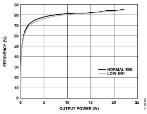
Figure 55. Efficiency vs. Output Power ( $P_{OUT}$ ),  $RL = 3 \Omega$ , No FB and 220 pF Capacitor,  $PV_{DD} = 12$  V, Analog Gain = 12.6
