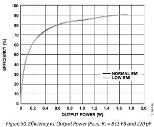
Capacitor,  $PV_{DD} = 5 V$ , Analog Gain = 6.3
