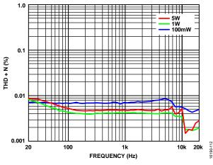
Figure 18. THD + N vs. Frequency into  $R_L = 8 \Omega$ ,  $PV_{DD} = 12 V$
