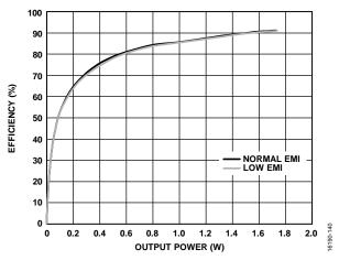
Figure 46. Efficiency vs. Output Power ( $P_{OUT}$ ),  $R_L = 8 \Omega$ , No FB and 220 pF Capacitor,  $PV_{DD} = 5 V$ , Analog Gain = 6.3
