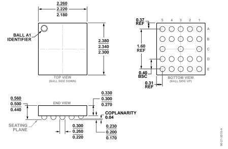
Figure 85. 23-Ball Wafer Level Chip Scale Package [WLCSP] (CB-23-2) Dimensions shown in millimeters
