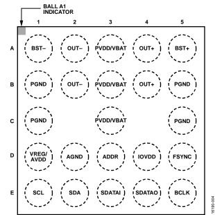
Figure 5. Ball Configuration (Top Side View)
