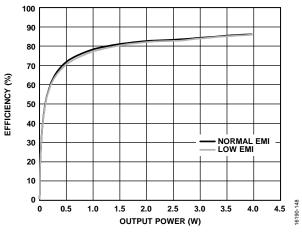
Figure 54. Efficiency vs. Output Power ( $P_{OUT}$ ),  $R_L = 3 \Omega$ , No FB and 220 pF Capacitor,  $PV_{DD} = 5 V$ , Analog Gain = 6.3
