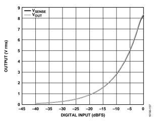
Figure 62. Voltage Sense Output vs. Amplifier Output  $V_{RMS}$ ,  $PV_{DD} = 12 V$ , Analog Gain = 12.6
