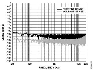
Figure 58. I/V Sense FFT, No Signal, PV<sub>DD</sub> = 12 V, Analog Gain = 12.6
