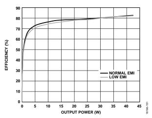
Figure 56. Efficiency vs. Output Power ( $P_{OUT}$ ),  $R_L = 3 \Omega$ , No FB and 220 pF Capacitor,  $PV_{DD} = 17 V$ , Analog Gain = 16
