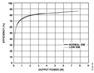
Figure. Efficiency vs. Output Power ( $P_{OUT}$ ),  $R_L = 3 \Omega$ , No FB and 220 pF Capacitor,  $PV_{DD} = 7 V$ , Analog Gain = 8.9
