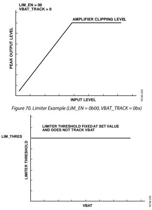
*Figure 71. Limiter Fixed (LIM\_EN = 0b01, VBAT\_TRACK = 0b0)*
