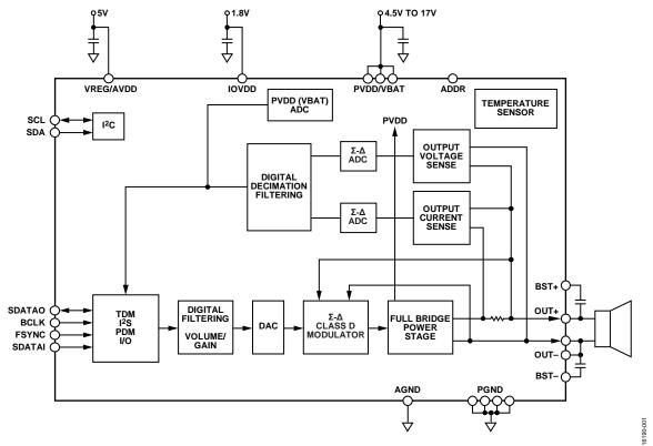
Figure 1. SSM3525 Block Diagram
