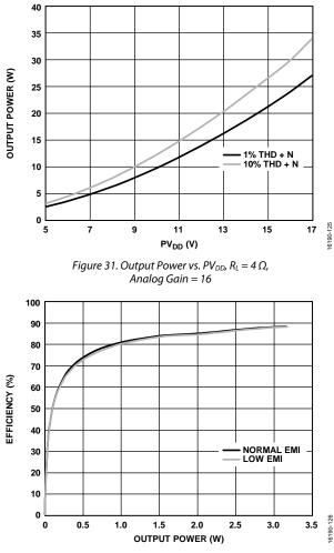
Figure 32. Efficiency vs. Output Power ( $P_{OUT}$ ),  $R_L = 4 \Omega$ , No Ferrite Bead (FB) and 220 pF Capacitor,  $PV_{DD} = 5 V$ , Analog Gain = 6.3
