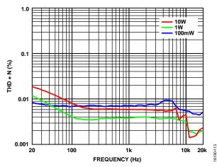
Figure 19. THD + N vs. Frequency into  $R_L = 8 \Omega$ ,  $PV_{DD} = 17 V$
