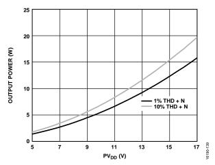
Figure 45. Output Power vs.  $PV_{DD}$  Supply Voltage ( $PV_{DD}$ ),  $R_L = 8 \Omega$ , Analog Gain = 16
