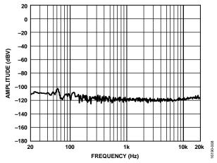
Figure 13. FFT, No Signal, Analog Gain = 16,  $R_L$  = 4  $\Omega$
