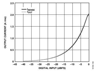
Figure 63. Current Sense Output vs. Amplifier Output Current Arms,  $PV_{DD} = 12 V$ , Analog Gain = 12.6
