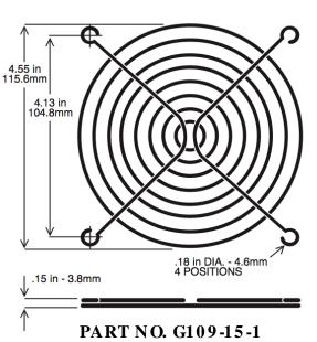
WIRE DIAMETER. RING DIA: 1.8 m m RIB DIA: 1.8 m m
