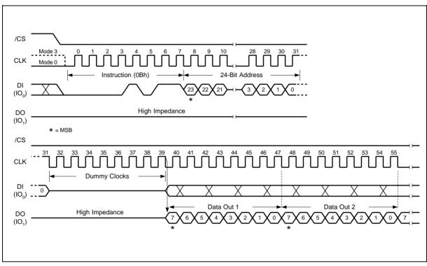
Figure 10. Fast Read Instruction Sequence Diagram
