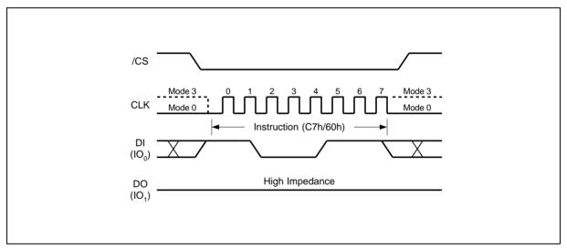
Figure 22. Chip Erase Instruction Sequence Diagram
