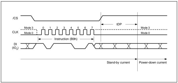
Figure 25. Deep Power-down Instruction Sequence Diagram
