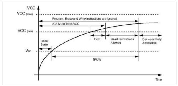
Figure 35a. Power-up Timing and Voltage Levels
