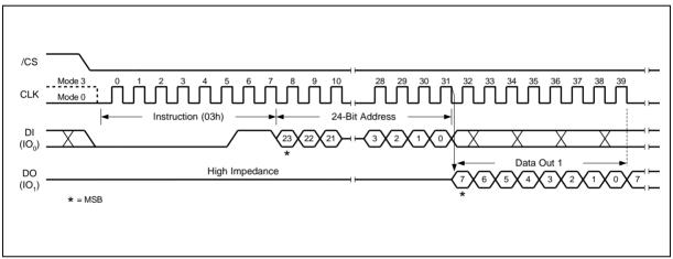
Figure 9. Read Data Instruction Sequence Diagram
