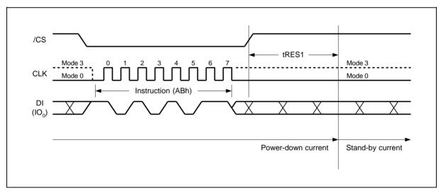
Figure 26a. Release Power-down Instruction Sequence
