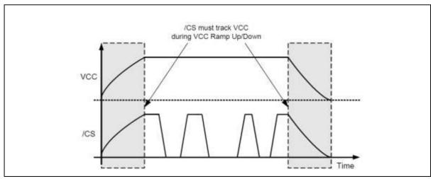
Figure 35b. Power-up, Power-Down Requirement
