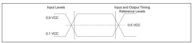
Figure 36. AC Measurement I/O Waveform
