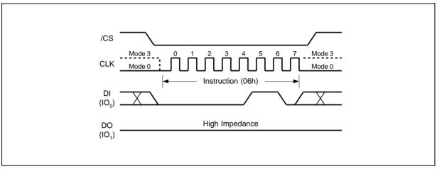
Figure 4. Write Enable Instruction Sequence Diagram
