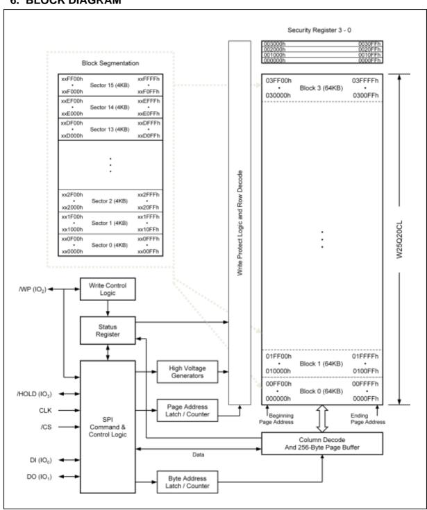
Figure 2. W25Q20CL Serial Flash Memory Block Diagram
