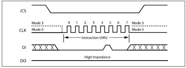
Figure 6. Write Disable Instruction Sequence Diagram
