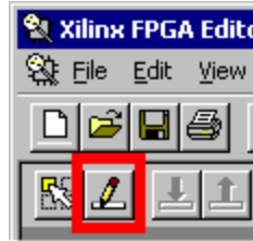
Figure 7: Click "Edit Mode" Button to Change DCM Settings
