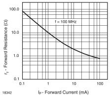
Fig. 1 - Forward Resistance vs. Forward Current
