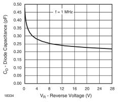
Fig. 2 - Diode Capacitance vs. Reverse Voltage
