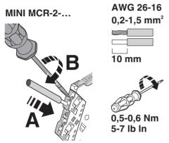
Figure 4 Screw connection
