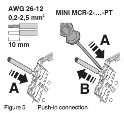
Insert the wire into the corresponding connection terminal block.
