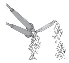
Figure 6 Test disconnect terminal block
