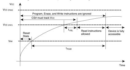
Figure 4.5 Power-Up Timing and Voltage Levels
