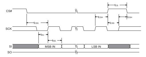
Figure 4.9 SPI Single Bit Output Timing
