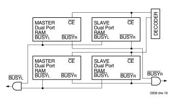
Figure 3. Busy and chip enable routing for both width and depth expansion with IDT7026 RAMs.
