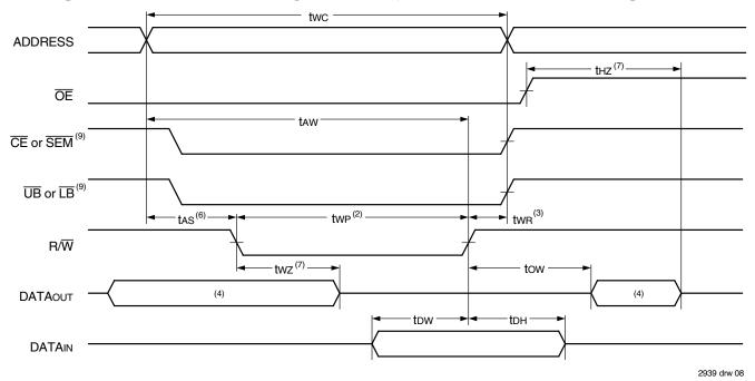
Timing Waveform of Write Cycle No. 2, CE, UB, LB Controlled Timing<sup>(1,5)</sup>
