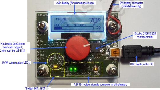
Figure 1: AS5134 Demoboard hardware with mounted magnet knob
