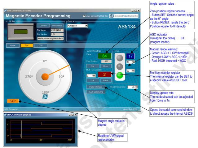
Figure 4: TWI tab, allows access to the AS5134 registers from the serial bus
