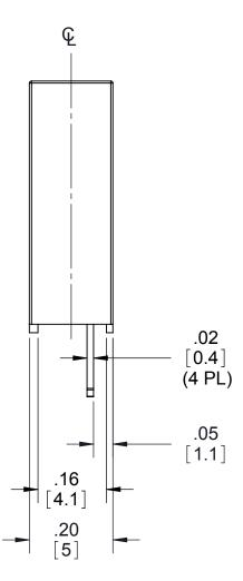
Tolerances: ± 0.02 in / 0.5 mm. All dimensions are in: inches [millimeters]
