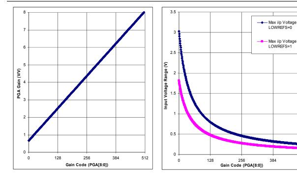
Figure 12 PGA Gain Characteristic
