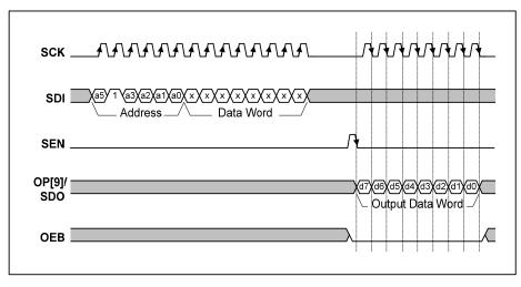
Figure 17 Serial Interface Register Read-back
