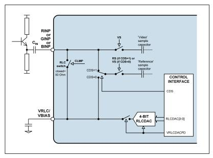
Figure 11 CDS/non-CDS Input Configuration
