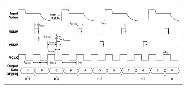
Figure 1 Three-channel CDS Input Video Timing (CDS=1)
