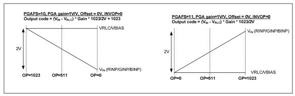
Figure 14 ADC Input Black Level Adjust Settings
