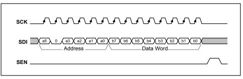
Figure 16 Serial Interface Register Write
