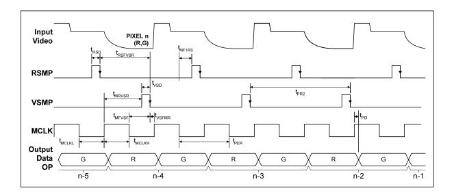
Figure 2 Two-channel CDS Operation (CDS=1)
