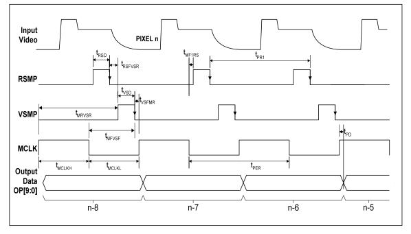
Figure 3 One-channel CDS Operation (CDS=1)
