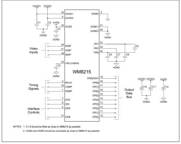
Figure 18 External Components Diagram
