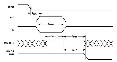
Figure 15. IDMA Address Latch
