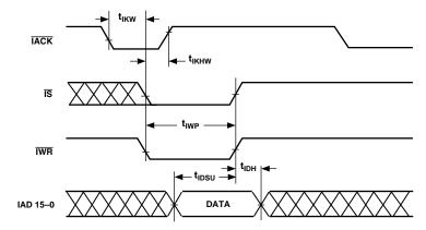
Figure 16. IDMA Write, Short Write Cycle
