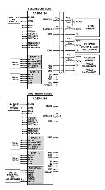
Figure 2. Basic System Configuration
