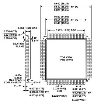
NOTE: THE ACTUAL POSITION OF EACH LEAD IS WITHIN (0.08) 0.0032 FROM ITS IDEAL POSITION WHEN MEASURED IN THE LATERAL DIRECTION. CENTER FIGURES ARE TYPICAL UNLESS OTHERWISE NOTED
