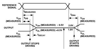
HIGH-IMPEDANCE STATE. TEST CONDITIONS CAUSE THIS VOLTAGE LEVEL TO BE APPROXIMATELY 1.5V.
