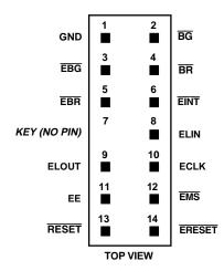
Figure 8. Target Board Connector for EZ-ICE
