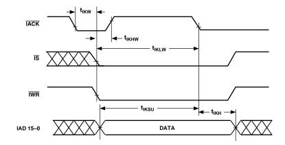
Figure 17. IDMA Write, Long Write Cycle
