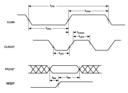
\*PF2 IS MODE C, PF1 IS MODE B, PF0 IS MODE A
