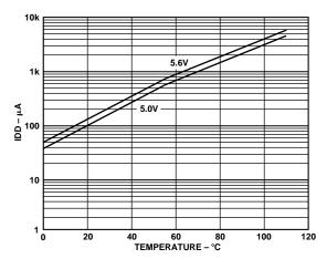
Figure 27. Power-Down Supply Current
