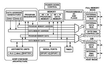
Figure 1. Block Diagram
