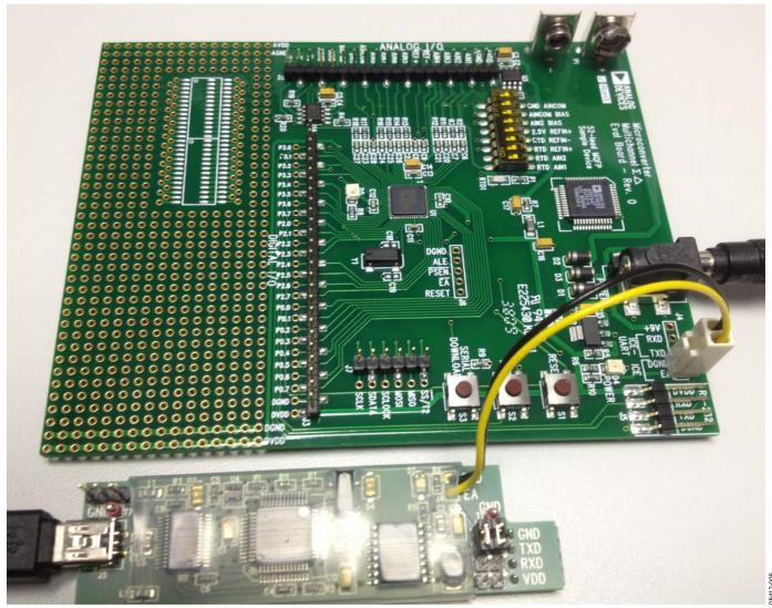
Figure 6. Target Board Connected to the USB-EA Emulator
