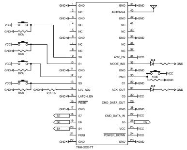
Figure 31: TT Series Transceiver Basic Application Circuit
