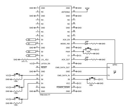
Figure 32: TT Series Transceiver Typical Application Circuit with External Microprocessor
