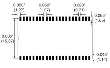
Figure 35: Recommended PCB Layout
