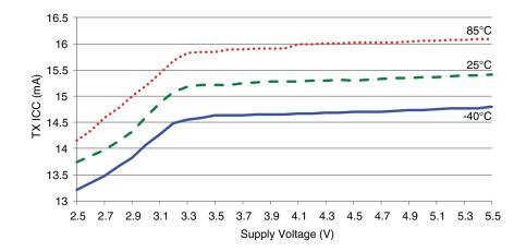
Figure 12: TT Series Transceiver TX Current Consumption vs. Supply Voltage at OdBm
