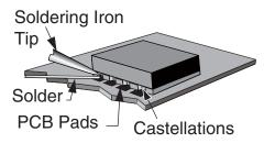
Figure 38: Soldering Technique
