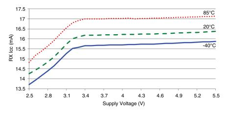
Figure 14: TT Series Transceiver RX Current Consumption vs. Supply Voltage
