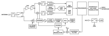
Figure 20: TT Series Transceiver RF Section Block Diagram
