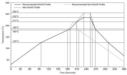
Figure 40: Maximum Reflow Temperature Profile
