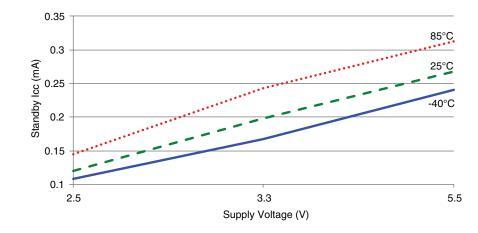
Figure 16: TT Series Transceiver Standby Current Consumption vs. Supply Voltage
