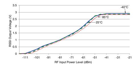
Figure 17: TT Series Transceiver RSSI Voltage vs. Input Power
