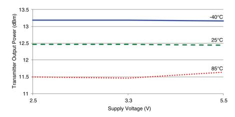
Figure 13: TT Series Transceiver Transmitter Output Power vs. Supply Voltage
