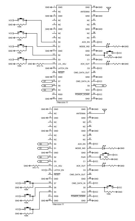
Figure 21: TT Series Transceiver Basic Application Circuits for Bi-directional Remote Control
